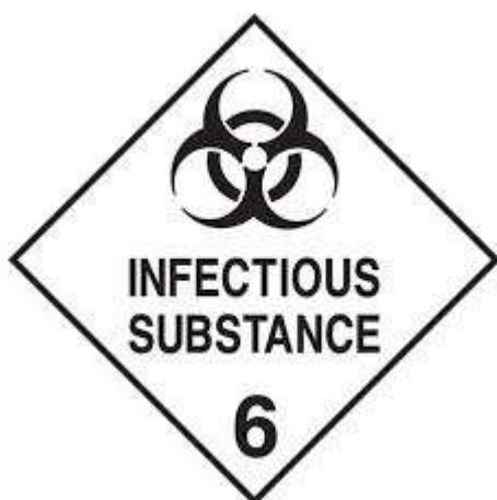
Figure 2: Class 6.2 Hazard Label for Transport
